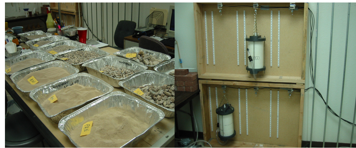
Photo 1. Different size fractions of test material
