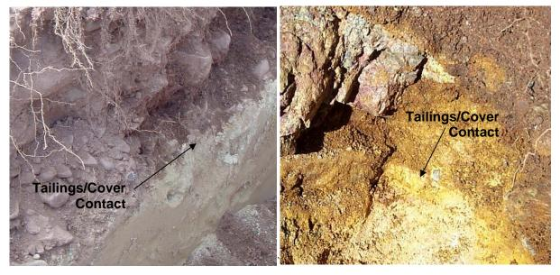
Figure 1. Typical tailings/cover contact in the Tailings 4W trenches on left, precipitate staining on above the tailings/cover system contact in the CTSA South Slope (right) area
