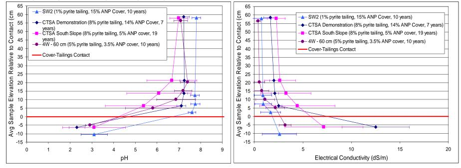
Figure 2. 1:1 Extract pH and EC vs depth interval in relation to tailings/cover contact for Tailings SW2, 4W, CTSA Demonstration and South Slope Areas
