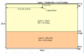
Figure 1. Model domain (Ks = Saturated Hydraulic Conductivity; bgs = below ground surface).
