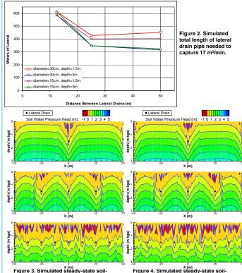
Figure 3. Simulated steady-state soilwater pressures for 15 cm diameter, 1.5 m bgs lateral drains at 50 m (top), 25 m (middle), and 12.5 m (bottom) spacing.
