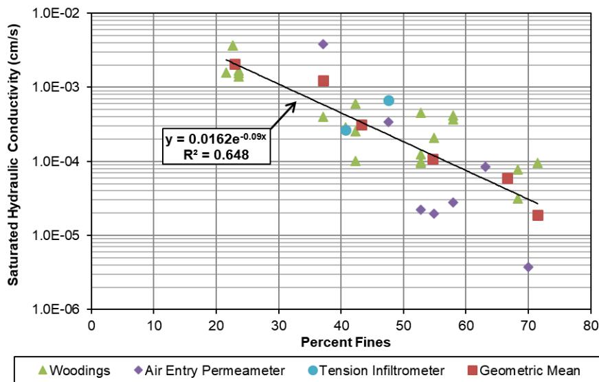
Figure 5. Tailings percent fines as a function of field measured saturated hydraulic conductivity.
