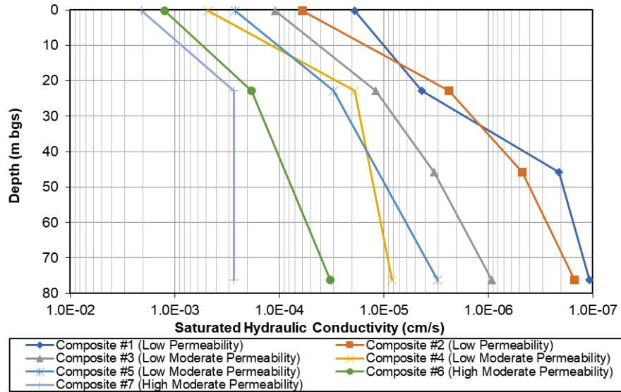
Figure 6. Saturated hydraulic conductivity as a function of tailings depth.
